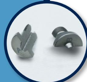
Divisible needle outlet. By this a perfect processing can be effected. Both halves for the needle outlet are manufactured through computer-controlling (CNC) and marked with A + B each. With several syringes, A + B always match.
