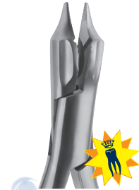
OLS-1332 DELPHIN Universal-Kramponzange Pin bending plier biegen/bending: max. .035" / 0,90mm schneiden/cutting: max. .028" / 0,7mm
