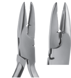
OLS-1333 WALDSACHS Universalzange Universal Pliers biegen/bending: max. .035" / 0,90mm schneiden/cutting: max. .028" / 0,7mm
